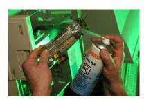
**FREEZER** is a rapid cooling agent for locating faults in electronic components and for cooling thermally sensitive parts during soldering or calibration.
