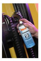
**CHAINSPRAY** is a lubricating and protective agent based on a mixture of oils, rust inhibitors and surfactants. It has been formulated to offer maximum adhesion to chain links for protection against rust, whilst also giving full penetration to lubricate the links.
