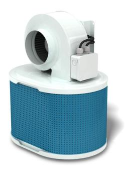
Designed for extraction and filtration of noxious fumes and vapours for the smaller workplace, for instance when soldering, gluing or working with solvents. It is intended to be used in different combinations with the FX arms or the Down Flow Grille FD 23. The fan and filter are ordered separatley unless included in a kit.
