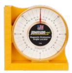
High-Impact molded body, Easy-to-read increments read 0-90 degrees in all four quadrants printed on durable acrylic lens, Extra-strong, ceramic magnet adheres to ferrous metal surfaces, V-Groove edge fits on pipe and conduit, Inch and metric graduations
