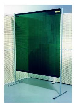
The protective curtain screens are easily movable for welding, grinding, turning, milling etc., and are ideal for the screening of temporary or permanent work places. The frame is manufactured from galvanised tube and the curtain of self-extinguishing PVC material and complying with EN 1598 for welding. Delivered complete with frame and curtain with total dimensions WxH=2000 x 2000 mm (just curtain H=1700 mm). Weight 7.5 kg.
