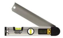
Digitally displays angle, Angle measurements in degrees, Working range of angle measurement 0 to 225°, Zero button for measurements of absolute or relative angles, Automatic shut-off after 5 minutes without use, 1750-1200 Includes > 1 3V CR2032 lithium battery, instruction manual.
