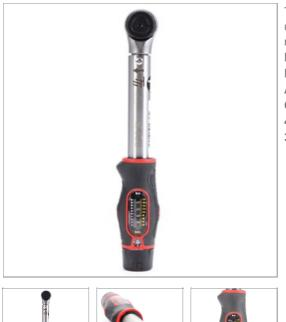
The Norbar TTi Torque Wrenches are accurate, easy to set and are comfortable in use. They are finished in an attractive and durable satin chrome plate. This TTi20 model is supplied with a 1/4" reversible ratchet. **Part number**: 13830 **EAN Bar Code**: 5060207563475 **NATO number**: 5120-99-344-4194 **Accuracy**: ±3% **Operates between**: 4.0 - 20.0 N·m **35.0 - 180.0 lbf·in**
