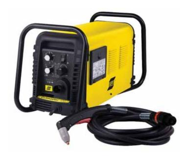
The ESAB Cutmaster 120, weighing only 28 kg and provides 120 amps of cutting power for a 40mm (1-1/2") recommended cut and 55mm (2-1/8") maximum cut. This compact unit, like all other Cutmasters, comes standard with the 1Torch® providing you with the well known comfort and reliability famous throughout the industry. Packages include power source, SL100 1Torch, spare parts kit, air filter/regulator, work cable and clamp and power cable.
