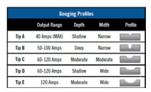
Gouging profile chart for choosing the right gouging tip based on your application
